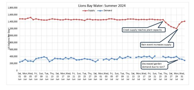
Rain passes through in 36-48 hours—we already see the curve flattening--and then we'll be back to steadily declining summer supply. With six months of leak detection bearing fruit, and knowing that we have a good response to Level 2 and Level 3 conservation, the municipality believes demand is well in hand. **We remain good at Level 1 conservation**, which only restricts lawn watering (to three days a week between 4 and 9 a.m.), with all other uses permitted.
